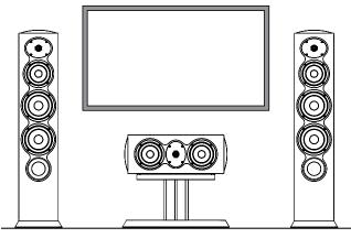
• When mounting the loudspeaker on the C Stand, if the speaker/ stand is placed more than approximately two feet (0.6m) from the front wall, set the C208's Low-Frequency Compensation Switch in the "Normal" position.
