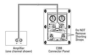
To make single-wired connections, connect one loudspeaker cable to the desired set of C208 input terminals. (The high-frequency — "HIGH" — input terminals are recommended.) Then connect the other end of that loudspeaker cable to the desired power amplifier output channel.
