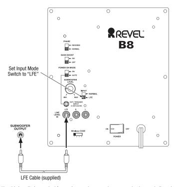
Use this installation method for receivers and preamps/processors that have a dedicated subwoofer output.
