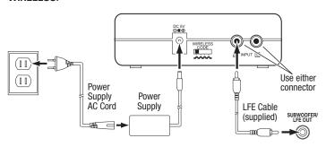
1. Connect the supplied LFE cable from your receiver's or processor's subwoofer output to either of the transmitter unit's Input connectors.
