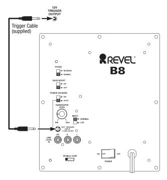
The subwoofer will automatically turn on if it receives a trigger voltage at its External Trigger Input connector and will enter the Standby mode when the voltage ceases.
