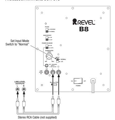
Use this installation method for receivers and preamp/processors that do not have a dedicated subwoofer output but do have preamp-level (volume-controlled) line outputs.
